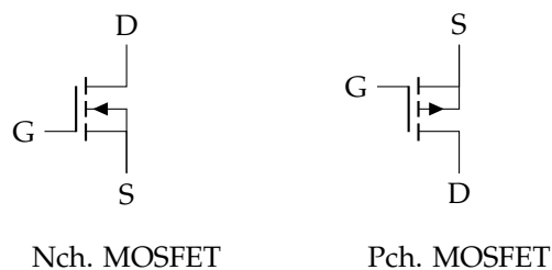
Fig. 2-2: Symbols of Enhancement MOSFET
